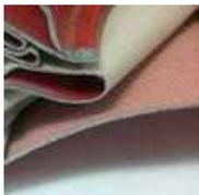
Tri-Poxy® coating lines the interior of all Chapin steel tanks (excluding stainless steel tanks). This photo shows the tank being crushed. Note that the coating did not crack, flake, or chip under the extreme stress on the metal.
